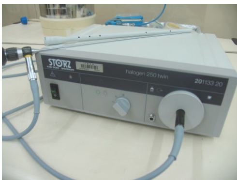
Figure 11 – Rigid Rod endoscope used in LIT's welding laboratory.
