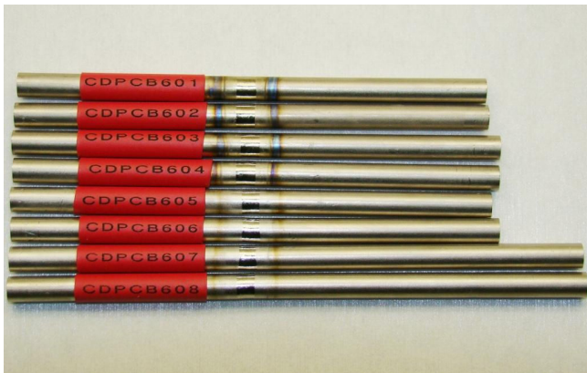
Figure 13 – Additional set of STBs for evaluation of late soldering after storage.
